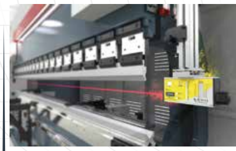
CE Laser Safety System
