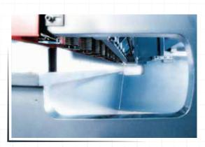
Special Throat Depth Throat depth of at least 350 mm allows the cutting of longer sheets than the knife length
